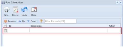
c. Place cursor on the **ID field**, the dropdown combobox button is shown. Click that button to bring down the combo box where rows to build the formula are shown. Select the row. The **Description field** will then show the description of the selected row.
