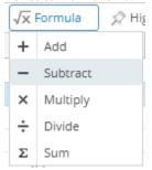
Example, the formula to build is R3 - R4. To build this, click on **Formula button** and select **Subtract**. A red broken line will be shown in the grid area.
